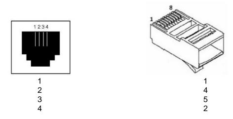
RJ11 Female to RJ45 Male Other Wiring Configurations Available
