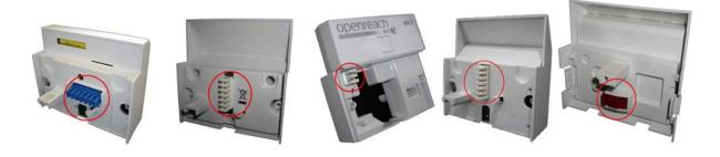
Terminate the BLUE pair to these terminals using the IDC tool provided. Solid BLUE goes to "A" BLUE/WHITE goes to "B".
